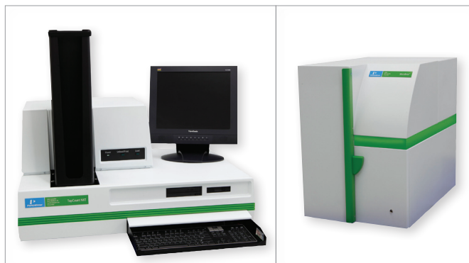
Figure 18. Left: TopCount NXT Microplate Scintillation Luminescence Counter; Right: MicroBeta 2 Plate Counter.
