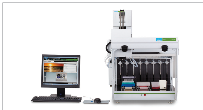
Figure 24. Automate small scale protein purification with the JANUS BioTx Pro Workstation.
