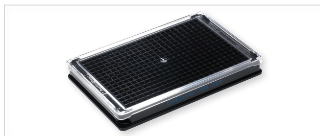
Figure 17. CellCarrier Ultra in a 384-well format.
